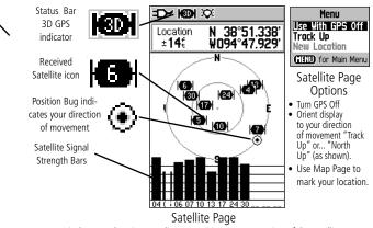
Displays your location coordinates, position accuracy, a view of the satellites overhead, and a bar graph showing the signal strength of each overhead satellite.
