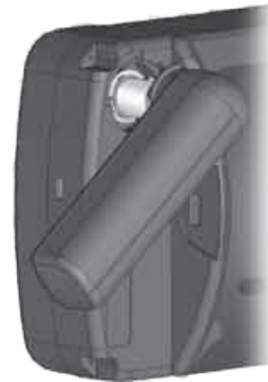
Removing the GPS Antenna
