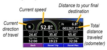
Touch **Reset Trip** to reset all information on the Trip Computer. To reset the maximum speed, touch **Reset Max**.
