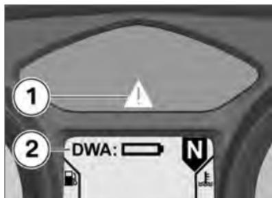
Anti-theft alarm warnings **2** appear in combination with 'General' warning light **1** showing after the Pre-Ride Check and relate to the capacity of the internal battery that supplies power to the anti-theft alarm.
