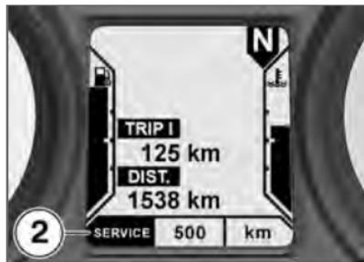
If the motorcycle covers long distances in the course of the year, under certain circumstances it might be necessary to have it serviced at a date in advance of the forecast due date. If the countdown distance to the odometer reading at which a service will be due is less than 1000 km, the distance is counted down in steps of 100 km **2** and is shown briefly after the Pre-Ride Check completes.
