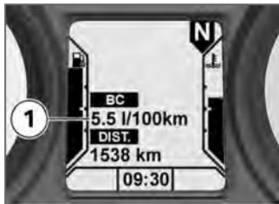
Average consumption **1** is calculated by dividing the distance covered since the last reset by the corresponding amount of fuel used.
