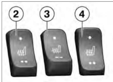
The rear seat has two-stage heating. Stage two is for heating the seat quickly: it is advisable to
