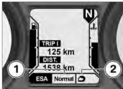
The selected riding mode is displayed in panel **1** of the multifunction display and the load status is displayed in panel **2**.
