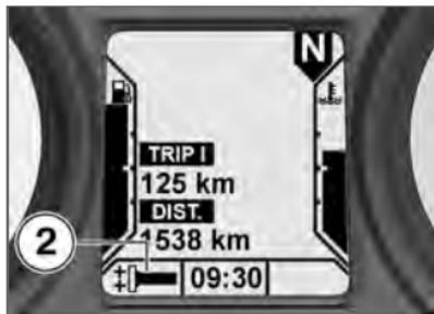
The handlebar grips have two-stage heating. Stage two is for heating the grips quickly: it is advisable to switch back to stage one as soon as the grips are warm. The heating stage you have selected is indicated by the symbol in the multifunction display **2**.
