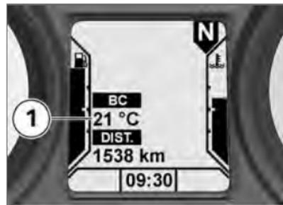
When the motorcycle is at a standstill the heat of the engine can falsify ambient-temperature reading **1**. If the effect of the engine's heat becomes excessive, – temporarily appears on the display.
