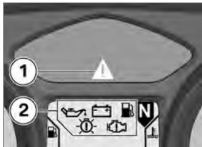
Warnings are indicated by 'General' warning light **1** showing in combination with one of the warning symbols **2**. The 'General' warning light shows red or yellow, depending on the urgency of the warning.
