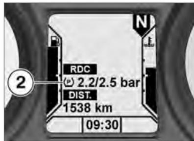
Tyre-pressure readings **2** are based on a reference tyre temperature of 20 °C. The front tyre pressure is on the left; the reading on the right is the rear tyre pressure. -- -- appears directly after the ignition is switched on, because the sensors do not transmit tyre pressures until the motorcycle accelerates to 30 km/h.<
