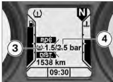
The tyre pressures for front wheel **3** and rear wheel **4** are shown. The graphic here indicates that the reading for the front wheel is flashing, which means that pressure in the front tyre has reached a critical value.
