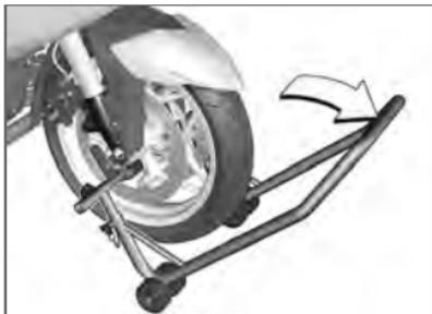
**!** If the motorcycle is on the centre stand and is raised too far, the centre stand will lift clear of the ground and the motorcycle could topple to one side. When raising the motorcycle, make sure that the centre stand remains on the ground.◀
