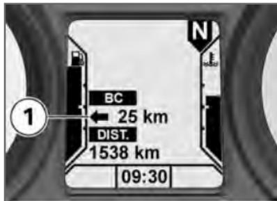
The description of the residual-range function (→ 52) also covers range readout **1**. You can also view the range before the fuel level drops to reserve.
