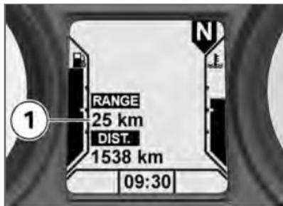
The residual-range readout **1** indicates how far you can ride with the fuel remaining in the tank. This reading is not displayed until fuel level has dropped to reserve. This distance is calculated on the basis of fuel level and average consumption.
