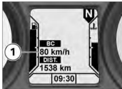
Average speed **1** is calculated on the basis of the time elapsed since the last reset. Times
