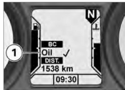
Oil-level indicator **1** gives you an indication of the engine oil level. You can call up this reading only when the motorcycle is at a standstill.
