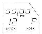
**PROGRAMMING -** When the total time of stored tracks exceeds 99m 59s '0000' is displayed. Further tracks can still be stored.
