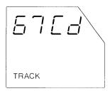
**ON** - As soon as the player is switched on, with the disc drawer empty, the display shows '67CD' briefly and then '- - - ' appears continuously (see **STANDBY** below). If a disc is in the drawer then after '67CD' the display shows the disc contents (see **PLAYING TIME** below).
