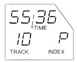
**PROGRAMMING** - When tracks are stored during programming a 'P' is displayed after the track number. Also the total additive playing time of all the selected tracks.
