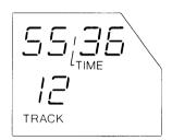
**PLAYING TIME -** When the contents of a disc have been read the highest track number is indicated together with the total playing time in minutes and seconds.
