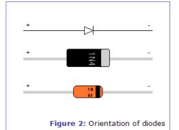
The cathode will be indicated by a white, silver or black line on the body of the diode.
