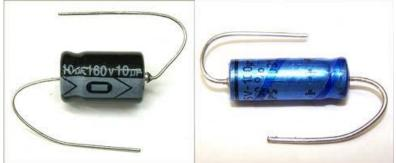
With axial capacitors there is an extra arrow indicating the minus wire, or there is a printed small ring around the body indicating the minus wire. Also the minus wire is direct connected to the aluminum body. The plus wire is sticking through the black plastic cap. **Indication of the cathode of diodes and zener diodes**
