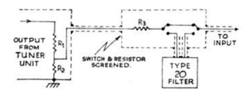
RESISTOR R1. Suitable value as load for tuner unit.
