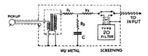
The transformer ratio should be chosen to provide 0.1 to 0.2 v.r.m.s. across the secondary, but the secondary impedance should not exceed 250,000 ohms. Should the pick-up already supply 0.1 v.r.m.s. then the transformer should be omitted.
