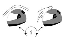
This picture shows the wind noises. If one helmet is in a streamlined flow (see left helmet) the wind noise will be equally constant and - in high quality helmets - rather muted. These conditions can mostly be found on 'naked bikes' or on bikes with minimal panels and small, flat windscreens. Under these conditions the intercom's automatic can easily tell wind noise outside the helmet from talk within the helmet. In this case the best position of the switch will be between 8 and 12 o'clock.
